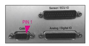
Note: Termination resistor between CAN-high and CAN-low is not installed.
