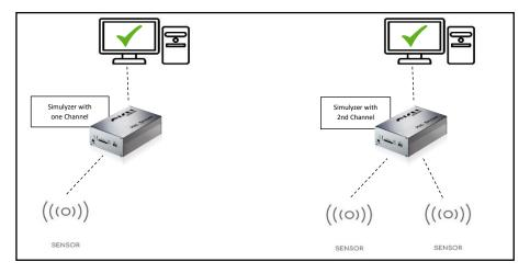
If you have bus connections or synchronous sensors, you can connect up to 12 sensors to one Simulyzer. The following setup shows you your configuration:
